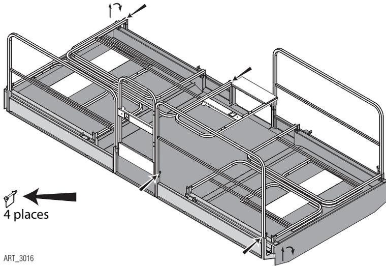
**4** Remove the safety snap pins from main deck rail panels that attach to the entry gates.
