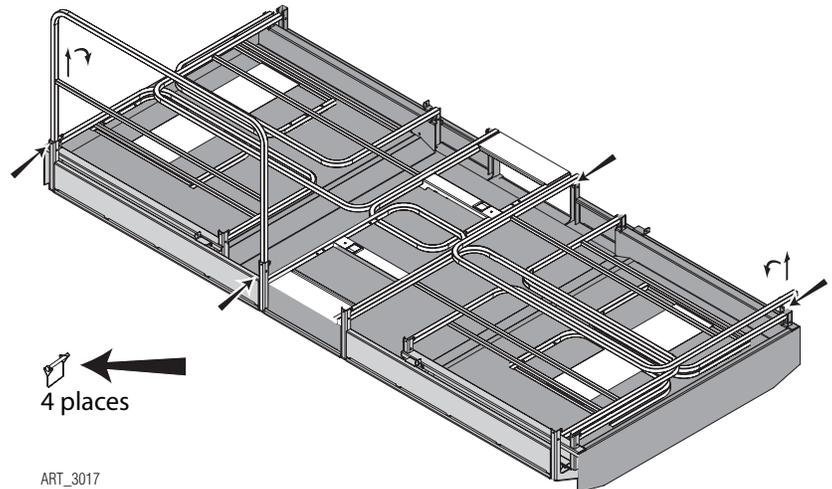
To return the machine to normal operation mode, lift all rails into their upright position, install all safety snap pins, and position the platform control box on the extension rail.
