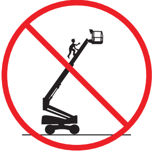
DO NOT ENTER OR EXIT PLATFORM WHEN ELEVATED
