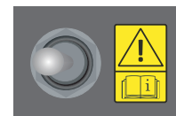
Emergency Platform Bypass Switch
