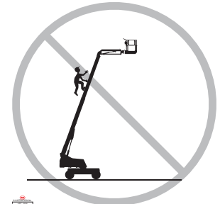
DO NOT ENTER OR EXIT PLATFORM WHEN ELEVATED
