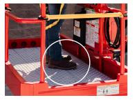
No footswitch required – allows the operator to position for maximum visibility whether driving or positioning the boom.
