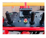
Proportional, multi-function controllers with secondary guarding to prevent crushing.
